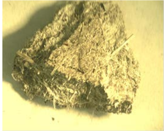
Cement based sheeting with white asbestos.
